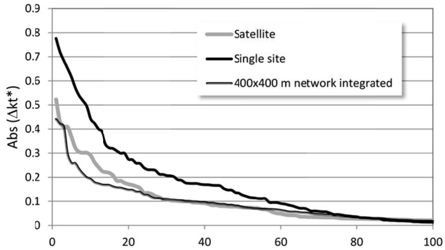
Fig. 4: Comparing satellite-derived and measured sorted absolute ramp rates at the Cordelia Junction network site
