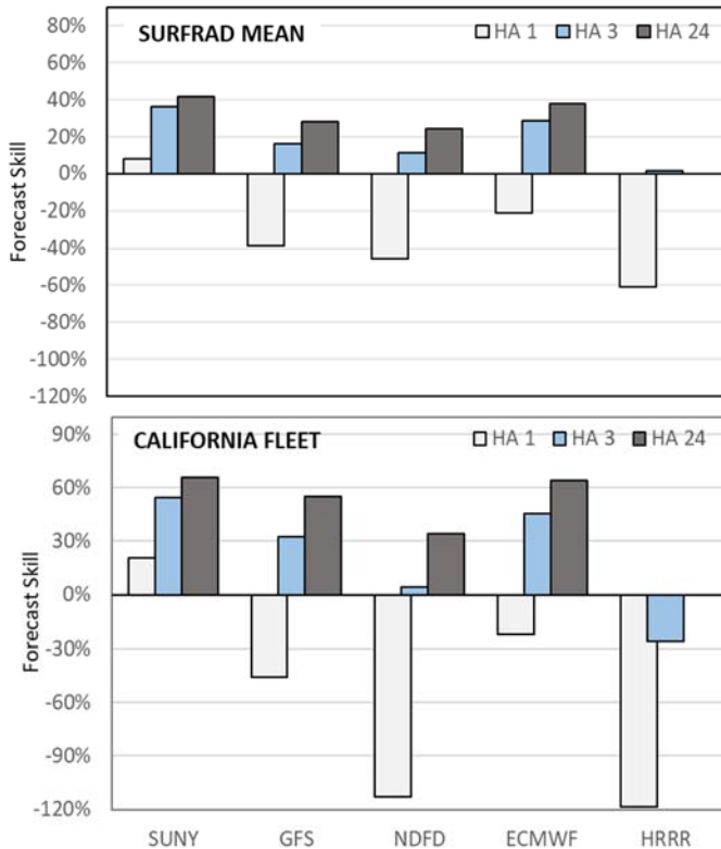
Fig. 3. Mean forecast skill for individual SURFRAD locations (top) and for the California Fleet (bottom)
