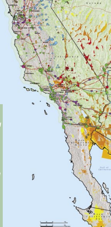
Figure 3. Direct-normal solar radiation maps – filtered by solar resource, topography, and land availability – identify the most economically suitable lands available for deploying large-scale concentrating solar power plants in the southwestern United States.
