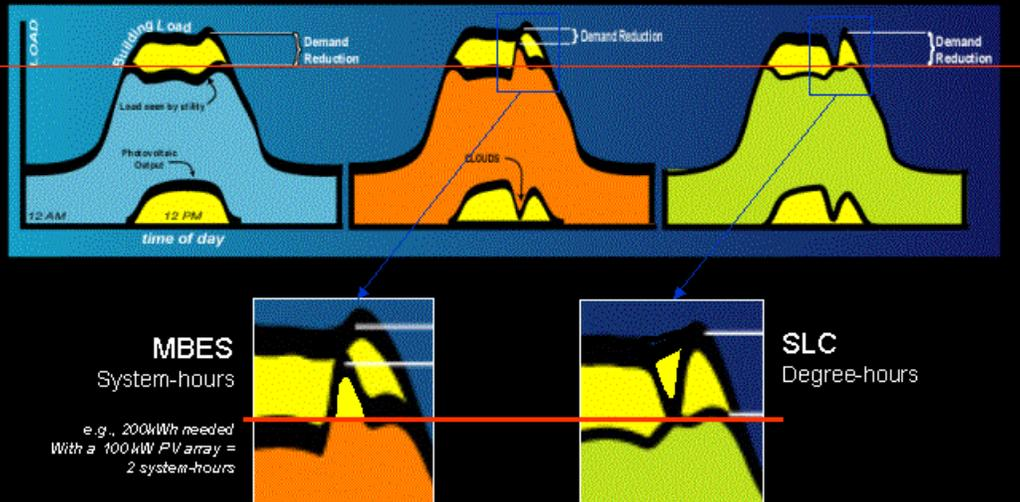
Sometimes conditions are not as ideal, so we looked at how much backup energy would be needed (middle diagram), or alternatively, how much end-use load control, i.e., consumption reduction, would be needed (right diagram), to guarantee that all resources above the red line are met.
